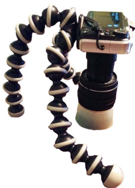
Figure A-5. Camera apparatus for imaging frozen particles.
