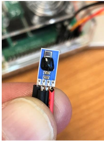
Figure 5. An HTY271 embedded water vapor and temperature sensor after harness attachment.
