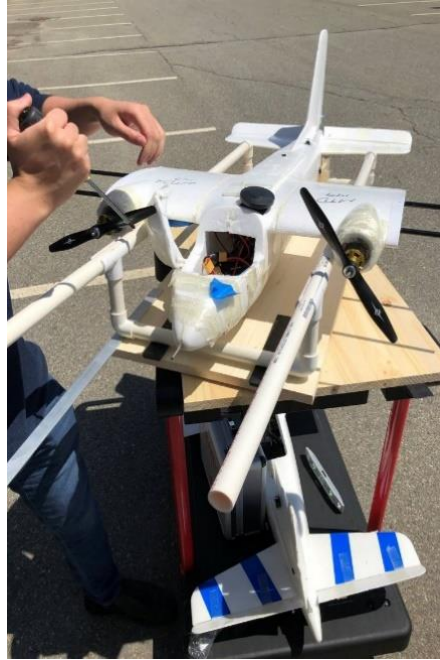
Figure 1. Magnetometer calibration testing on custom turntable.
